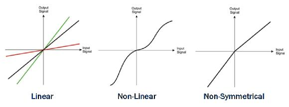
Fig. 4. Amplitude response graphs Input signal vs. Output Signal
